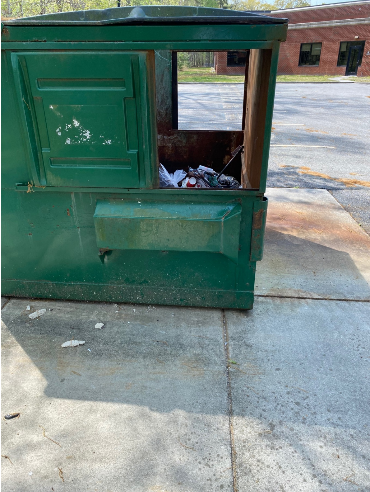
Photo #OF-G-3. Staining apparent on pavement all the way to receiving inlet (see also 2019-2020 report for this outfall). Staining indicates leak(s) in the bottom of dumpster. Dumpster also observed to be open, allowing for exposure of contents to stormwater.
